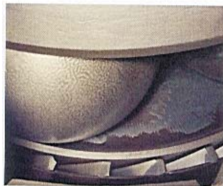
Self cleaning grinding mechanism avoids product build-up
